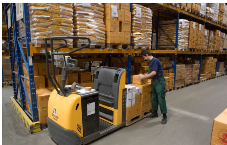
Figure 2 – Storage and order-picking system with selective pallet racks
